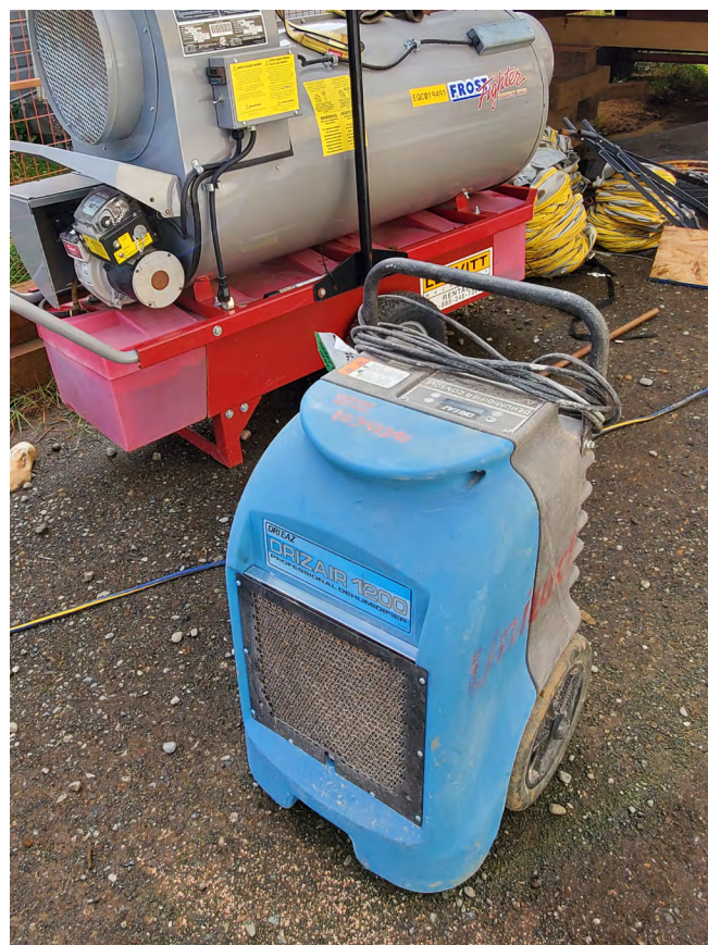
Figure 70 Heater and dehumidifier used in response to a moisture exposure event.
