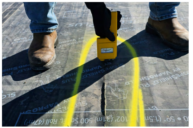
Figure 68 Moisture content reading taken at area of membrane damage.
