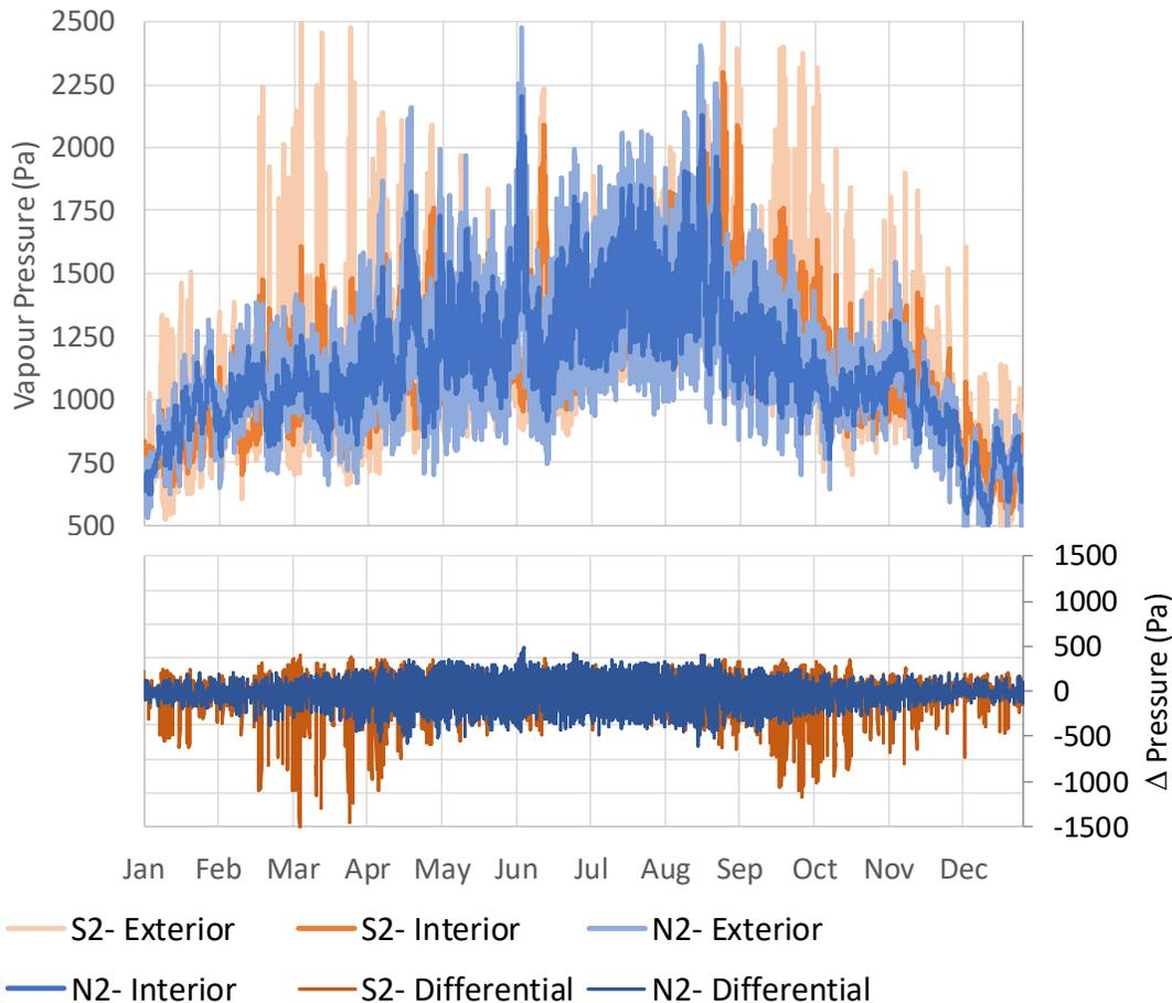
Figure 8: Cellulose Insulation Vapour Pressure and Vapour Pressure Gradients, for North and South Walls on Level 2.
