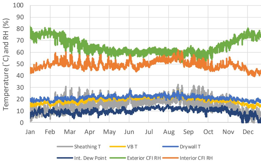
Figure 6: S2 wall data for Sheathing, Vapour Barrier (VB) and Drywall temperatures, including indoor air dew point temperature, and the exterior/sheathing and interior cellulose fibre insulation (CFI) relative humidity from January to December, 2016.
