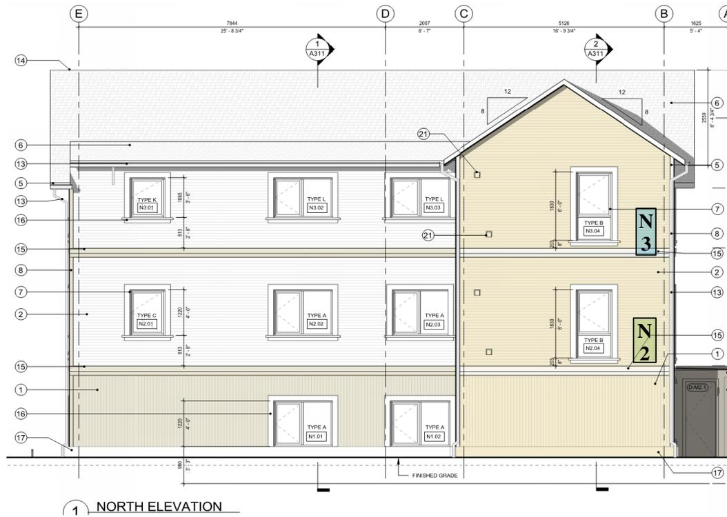
Figure 1: North elevation showing approximate locations for the instrumented enclosure sections.<sup>1</sup>
