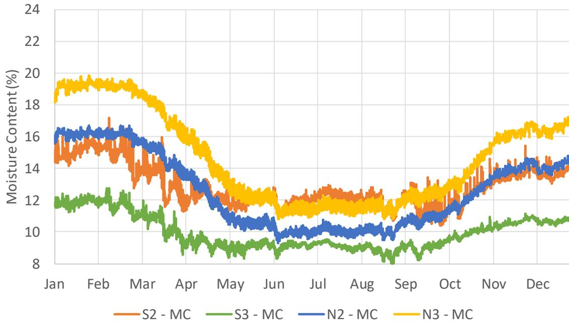
Figure 9: Sheathing Moisture Content (MC) for North and South Walls, on Levels 2 and 3.
