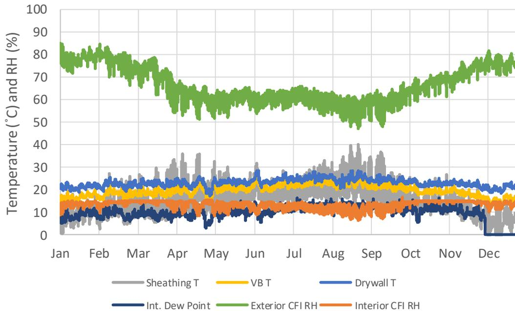
Figure 7: S3 wall data for Sheathing, Vapour Barrier (VB) and Drywall temperatures, including indoor air dew point temperature, and the exterior/sheathing and interior cellulose fibre insulation (CFI) relative humidity from January to December, 2016. The Interior CFI RH sensors is malfunctioning.
