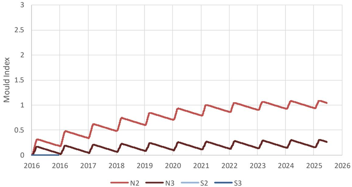
Figure 11: Maximum Supportable Mould Conditions for North and South Walls on the 2<sup>nd</sup> and 3<sup>rd</sup> Storeys
