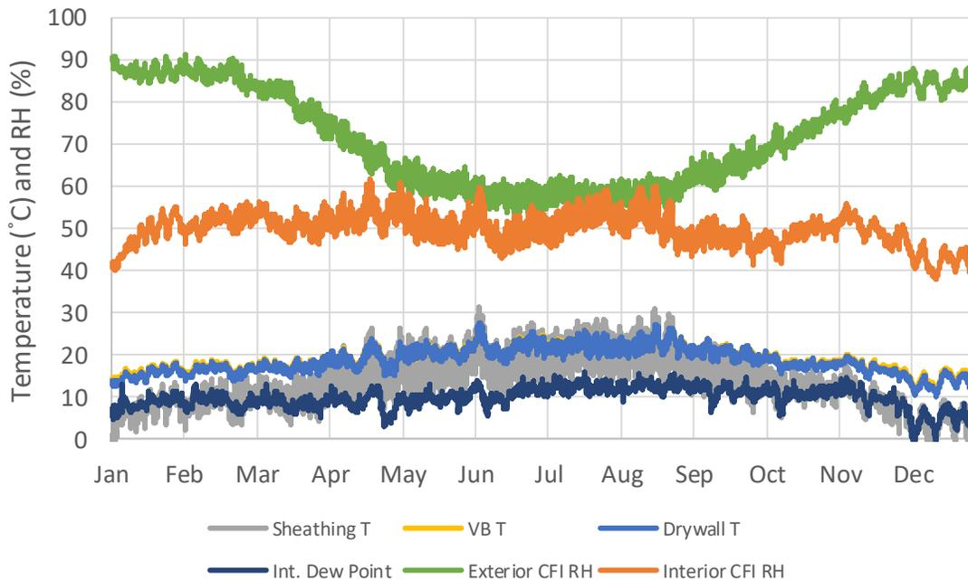
Figure 4: N2 wall data for Sheathing, Vapour Barrier (VB) and Drywall temperatures, including indoor air dew point temperature, and the exterior/sheathing and interior cellulose fibre insulation relative humidity from January to December, 2016.
