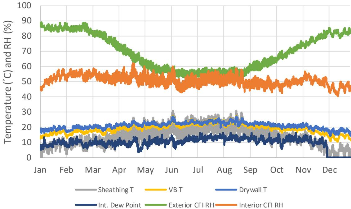
Figure 5: N3 wall data for Sheathing, Vapour Barrier (VB) and Drywall temperatures, including indoor air dew point temperature, and the exterior/sheathing and interior cellulose fibre insulation (CFI) relative humidity from January to December, 2016.
