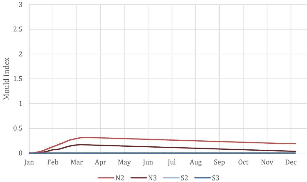
Figure 10: VTT Mould Index for N2, N3, S2, and S3 walls
