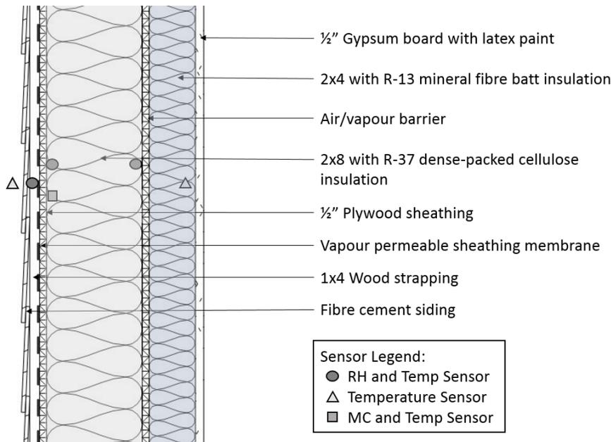
Figure 3: Detailed assembly and typical monitoring locations
