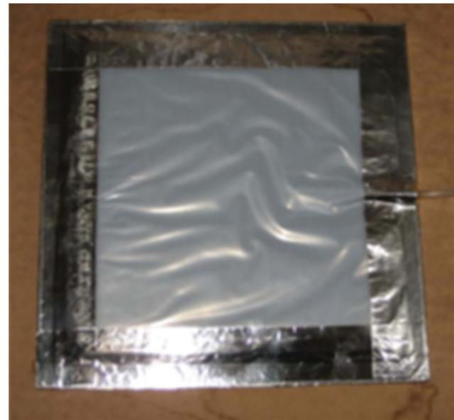
**Figure 3** Interior surface of subassembly test sample with interior wetting.
