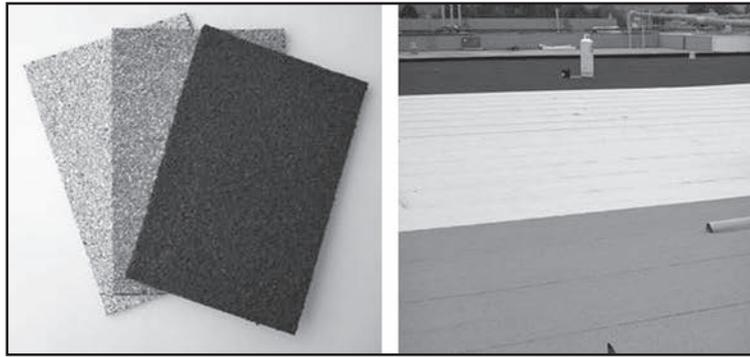
**Figure 5 – Membrane cap sheet colors (white, gray, and black) shown on left in lab (unsoiled and new) and shown on right in field shortly after installation.**
