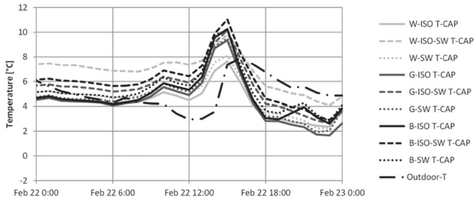
**Figure 11 – Roof membrane cap sheet temperature for nine monitored roof assemblies – Feb. 22, 2013 (winter).**
