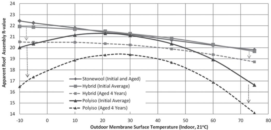
**Figure 7 – Apparent R-values of study building roof assemblies based on roof membrane surface temperature over a range of -10°C to 75°C (14°F to 167°F) (Dell and Finch, 2013).**
