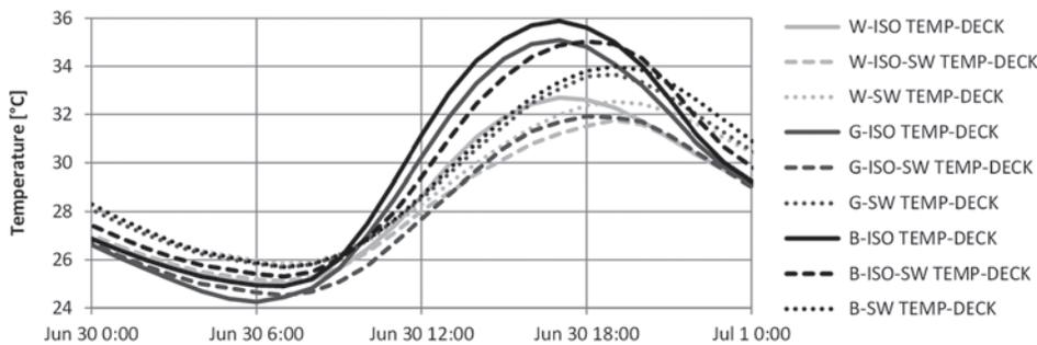
Figure 16 – Interior metal roof deck surface temperature for nine monitored roof assemblies – June 30, 2013 (summer).
