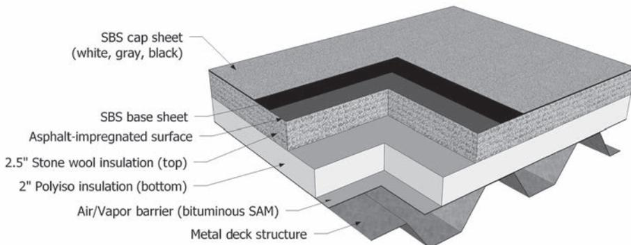
**Figure 4 – Hybrid roof assembly (2.5 in. stone wool over 2-in. polyisocyanurate, R-21.3); weight: 14.3 kg/m<sup>2</sup>, heat capacity: 13.7 kJ/K/m<sup>2</sup>.**
