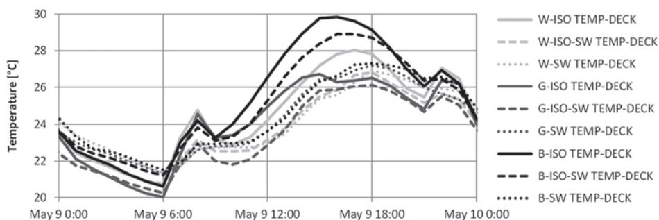
**Figure 14 – Interior metal roof deck surface temperature for nine monitored roof assemblies – May 9, 2013 (spring).**
