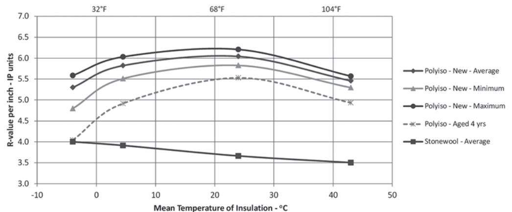
**Figure 6 – Apparent R-value per inch vs. mean temperature for polyisocyanurate and stone wool insulation (Dell and Finch, 2013)**
