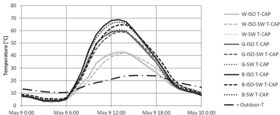
**Figure 13 – Roof membrane cap sheet temperature for nine monitored roof assemblies – May 9, 2013 (spring).**
