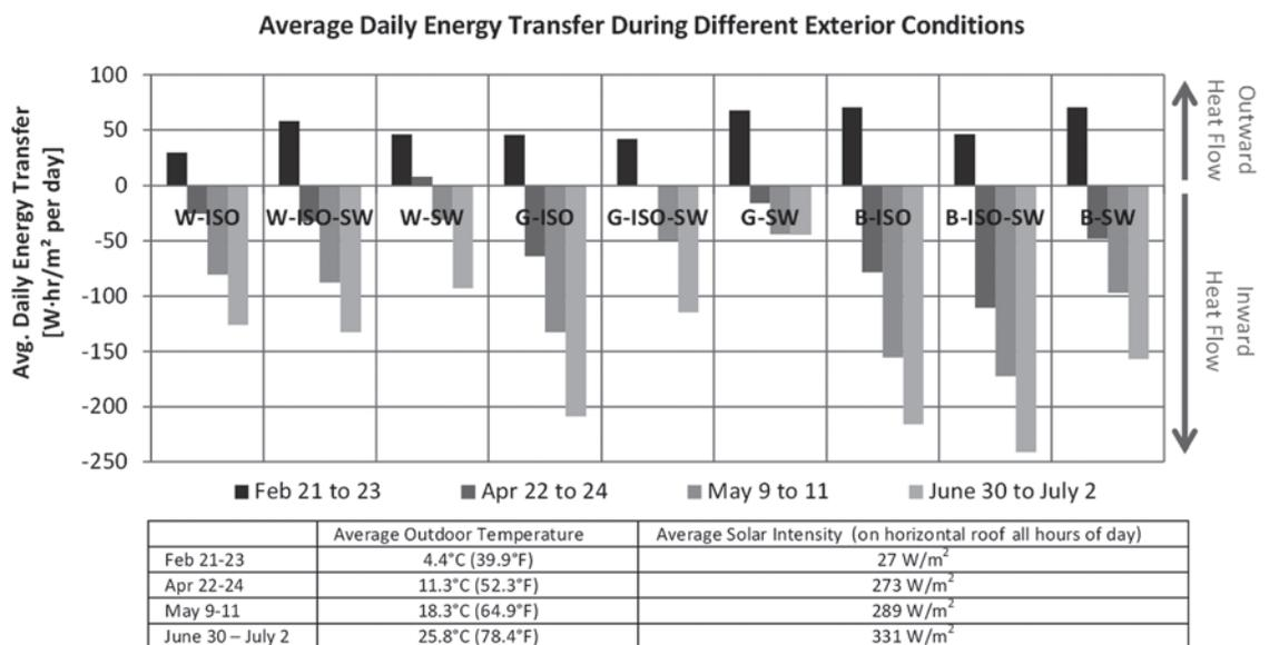
**Figure 10 – Heat flux measurements through each roof assembly – May 9-11, 2013 (spring warm) and June 30 – July 2, 2013 (summer peak design). Note: Data missing for G-ISO-SW for April 22-24 period and potentially inaccurate G-ISO and G-ISO-SW data for May 9-11 and June 30-July 2. White and black data for all three insulation materials are, however, accurate and representative of monitored conditions.**
