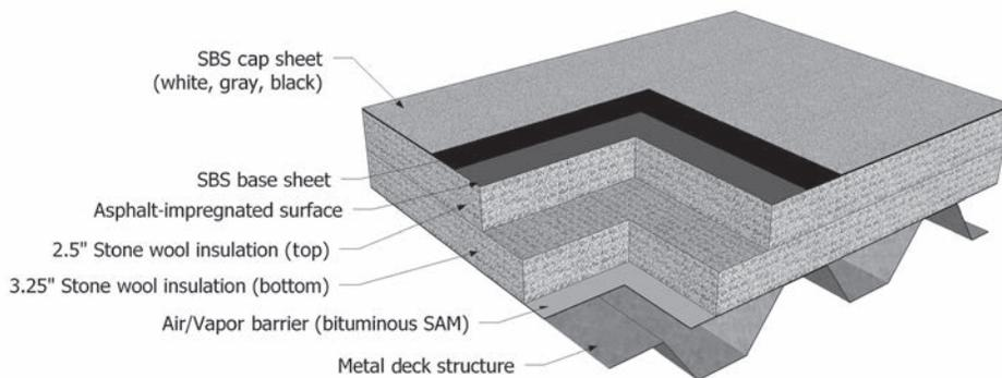
**Figure 3 – Stone wool roof assembly (5.75 in. stone wool, R-21.4); weight: 26.7 kg/m<sup>2</sup>, heat capacity: 22.7 kJ/K/m<sup>2</sup>.**
