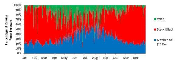
FIGURE 12: Graph of proportion of total absolute pressure difference attributable to each of the driving forces at the top of a 40 m tall building in Fairbanks
