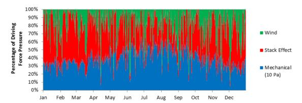
FIGURE 11: Graph of proportion of total absolute pressure difference attributable to each of the driving forces at the top of a 40 m tall building in Vancouver
