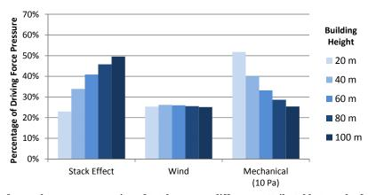
FIGURE 13: Graph of annual average proportion of total pressure difference attributable to each of the driving forces at the top of a building for various building heights in Vancouver
