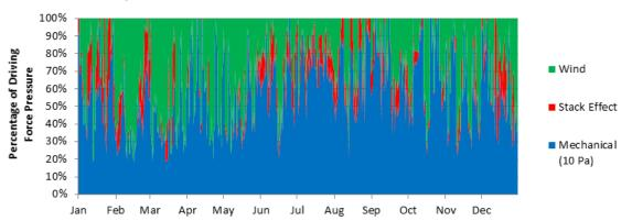
FIGURE 10: Graph of proportion of total absolute pressure difference attributable to each of the driving forces at the top of a 40 m tall building in Miami
