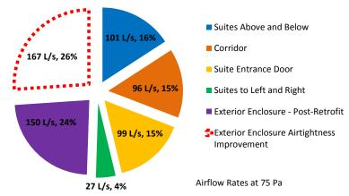
FIGURE 6: Chart showing the average distribution of airtightness for the tested suites
