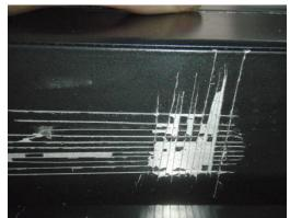
Figure 4: Cross-hatch pattern tested as outlined in AAMA 2604. This sample location is on a window frame member with chipped paint.
