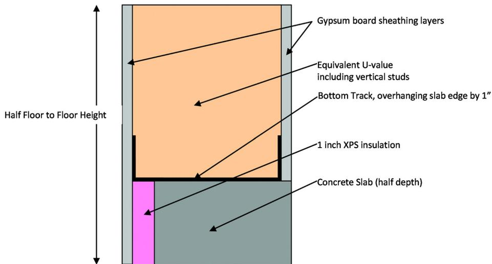
**Figure 4** Typical insulated slab edge: floor-to-wall section.
