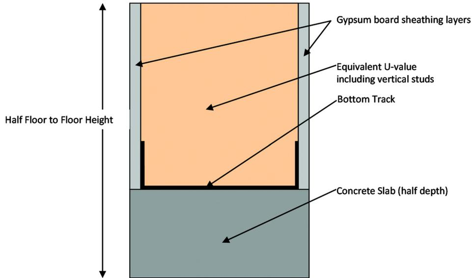
**Figure 3** Typical uninsulated slab edge: floor-to-wall section.
