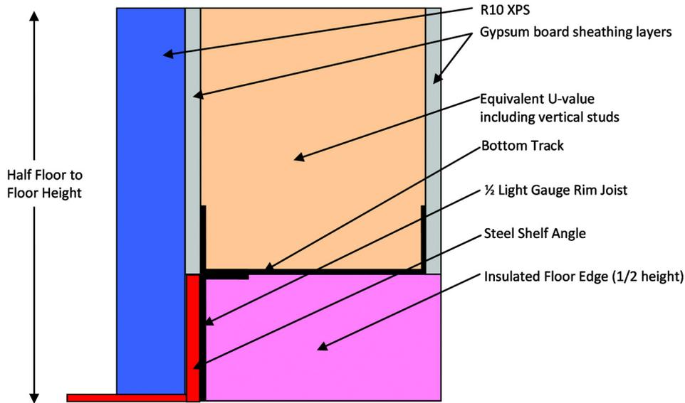
**Figure 5** Typical shelf angle at floor line.
