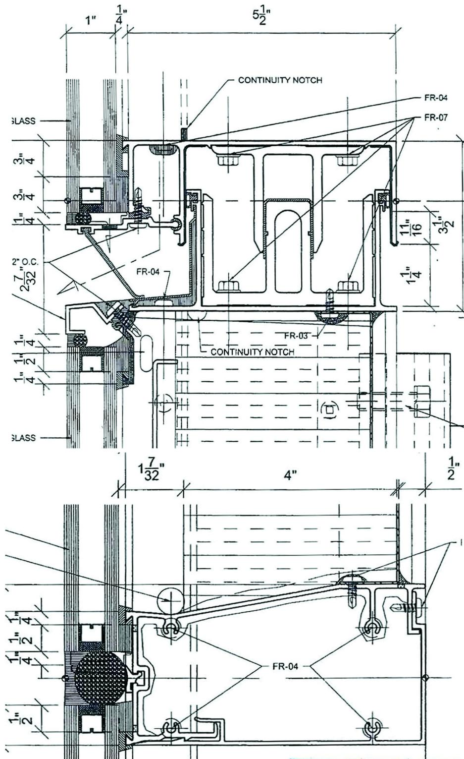
Figure 6 Curtain wall section.
